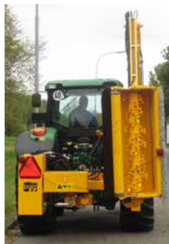
Back lights attached by magnet allow flexible use of lighting and can be used on all possible work tools.
