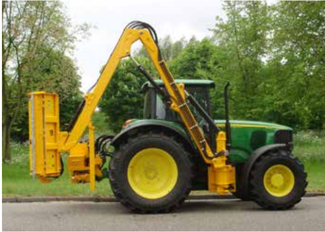
The Cavalier can be equipped optionally with long booms and rearward-facing transport position for better view during transport (MBK 418).
