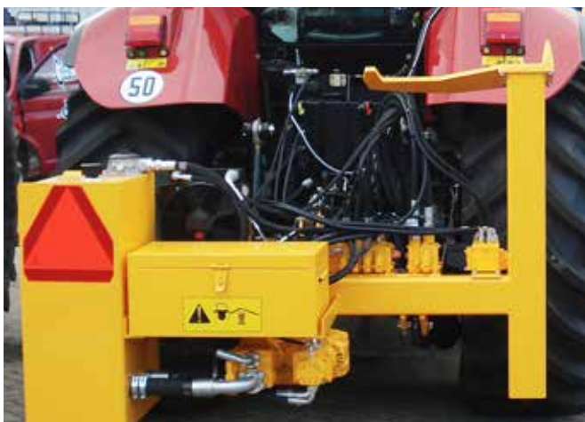
Simple but functional hydraulic unit carried in the 3-point linkage of the tractor, combined with a transport support on the back.
