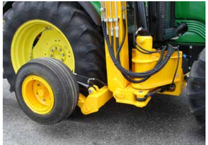
A support leg or support wheel is available for extra stability. A safe option, which also ensures even more job satisfaction.
