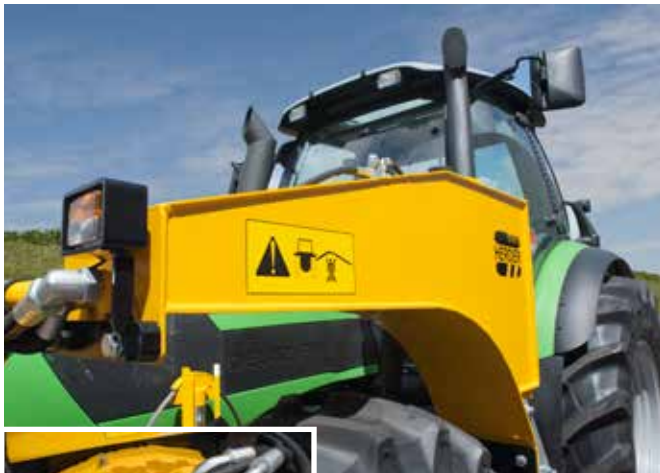
An example of a special version of the Cavalier. The pumps are connected to the front PTO and the hydraulic tank is placed above the left front wheel. In this model, the back lifting device and PTO remain available, for example for a side flail mower.
