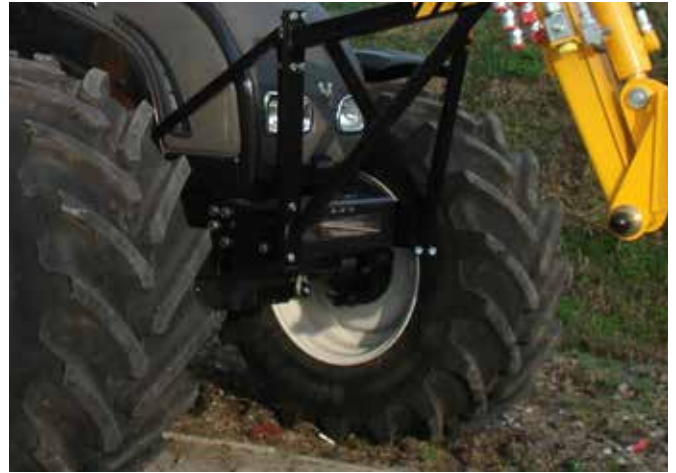
Work tool carrier on the front of the mounting frame. The boom rests on it in the transport position.
